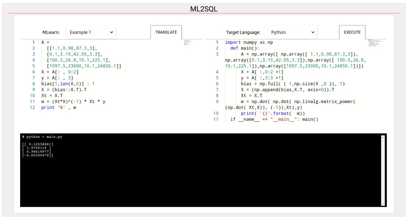
Figure 4: Web interface for an interactive exploration of the MLearn language: Above left, the text editor allows to specify tasks, which are translated into the selected target language (above right). The code will be executed in the terminal.
